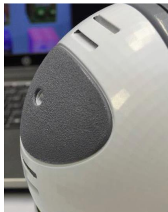
Figure 1.3 Up-close view of controller's grey textured oval pad and proximity sensor
